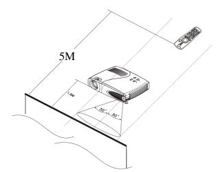
Users, using the remote control can, either point it directly at the IR Transceiver, or stand behind the unit and point it at the projected image.
